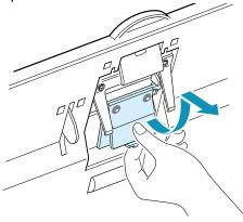
**3** Insert the tabs at the top of the new ADF rubber assembly into the slots and then push it down until it locks into position.
